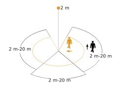
Possible mounting height: 2,00 m – 5,00 m Orange: radial Black: tangential 3 scalable zones
